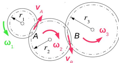
$$\rightarrow \omega_3 = \omega_2 \frac{r_2}{r_3} = \omega_1 \frac{r_1}{r_2} \frac{r_2}{r_3} = \omega_1 \frac{r_1}{r_3}$$
