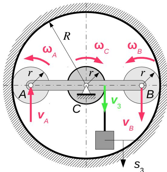
$$v_B = r \omega_B \rightarrow \omega_B = \frac{v_B}{r} = \left( \frac{R}{r} - 1 \right) \frac{v_3}{r} = \omega_A$$
