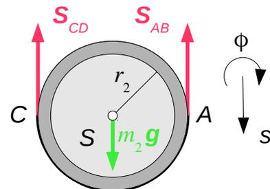
$$\begin{aligned} -S_{CD} - S_{AB} &= m_2(a - g) \\ S_{CD} - S_{AB} &= \frac{J_2}{r_2^2} a \end{aligned}$$
