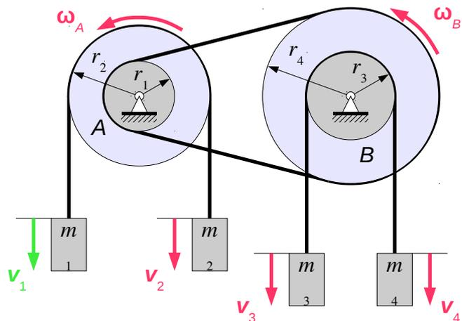
$$\rightarrow \omega_B = \frac{r_1}{r_4} \omega_A = \frac{r_1}{r_2 r_4} v_1$$
