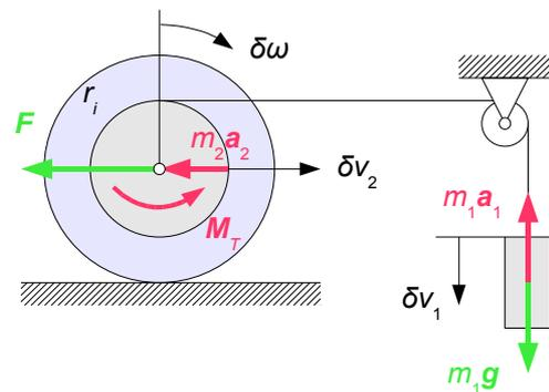
$$\frac{\partial F_2}{\partial s_1} \delta v_1 + \frac{\partial F_2}{\partial s_2} \delta v_2 + \frac{\partial F_2}{\partial \phi} \delta \omega = \delta v_1 - (r_a + r_i) \delta \omega = 0$$
