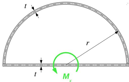
Zahlenwerte:  $r = 5 \text{ cm}$ ,  $t = 2 \text{ mm}$ ,  $M_x = 1200 \text{ Nm}$ ,  $R_m = 380 \text{ MPa}$ ,  $R_e = 235 \text{ MPa}$
